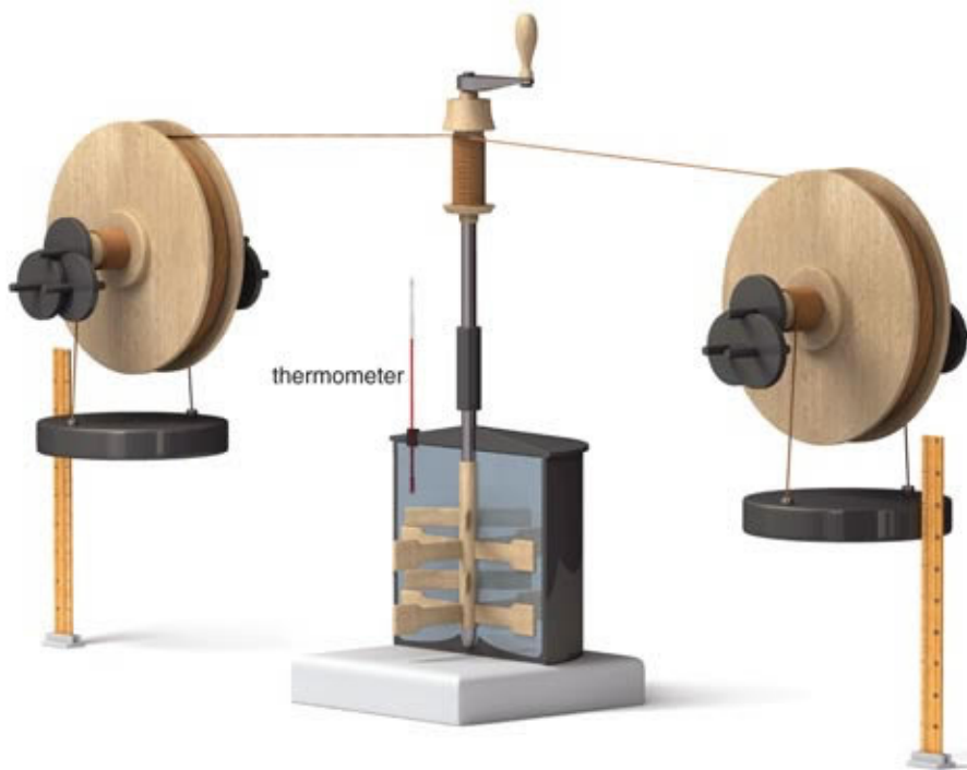
Figure 15.2 Apparatus for Joule's experiment on the mechanical equivalent of heat
