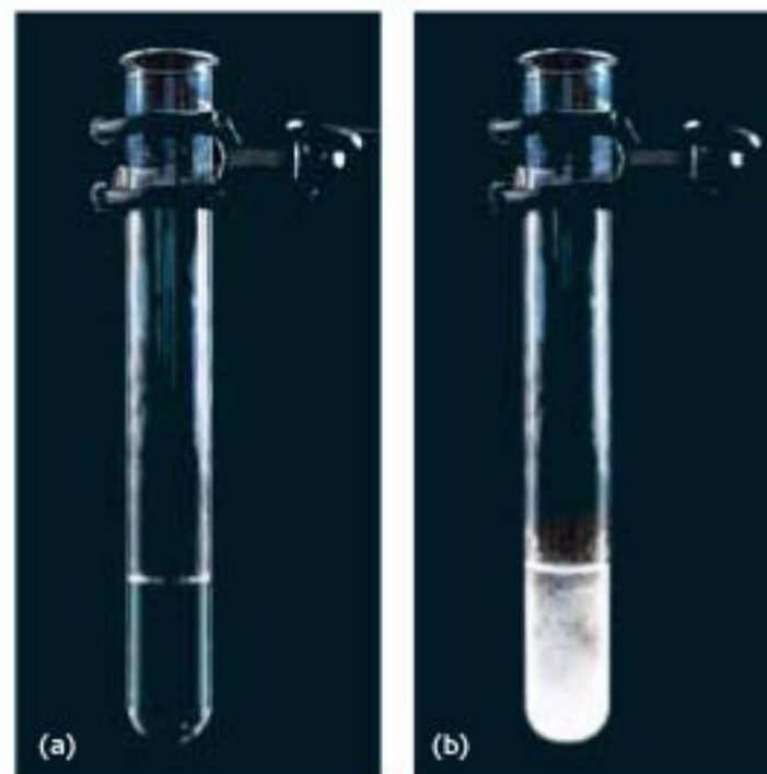
Figure 12.5 Crystallization of a supersaturated solution Addition of a “seed crystal” to a supersaturated solution of sodium thiosulfate (a) will cause the excess solute to crystallize (b), resulting in a saturated solution.
